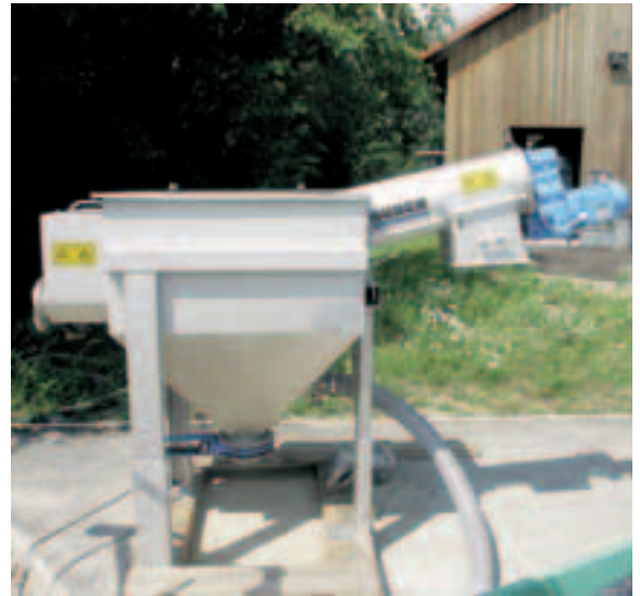
Mechanical preliminary MiniCop screen prior to HUBER BioMem®
