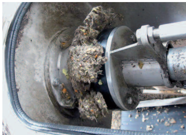
Discharge of the separated compacted material
