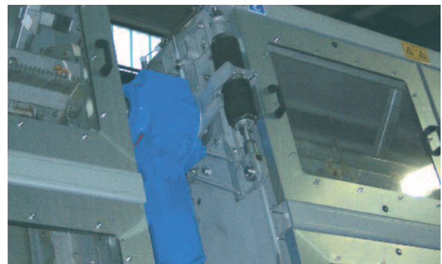
A control-independent safety system (torque compensator) reliably protects the screen against damage giving an electric signal. The specific design principle ensures high adjustability and continuous control.
